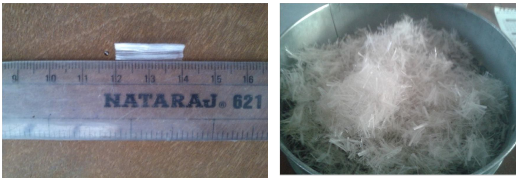
Fig 5 Fibrillated Polypropylene Fiber of 20mm Length
