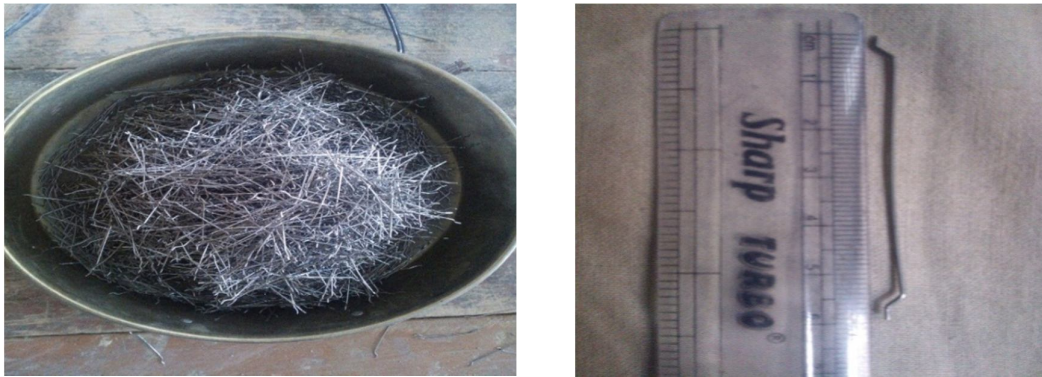
Fig 4 Steel fibers 60mm length hooked end with aspect ratio 75
